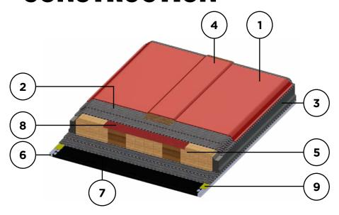
Lightness and power to hit the groomers and open fields of fresh pow. This construction uses multiaxial fiberglass, increasing its skiability and power by providing stiffness in torsion and flex. The goal was also to reduce the weight of these XXL skis, hence the combination or paulownia (lightness) and poplar (resistance). In the end, this construction creates a light and playful ski that's stable at high speeds and resistant over time!
