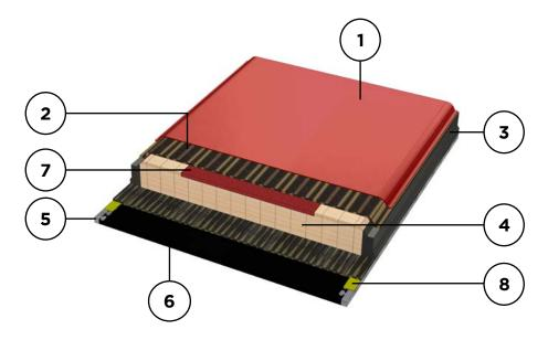
Built with the best ratio between lightness and skiability to give ski tourers the closest feeling to a freeride ski possible. The wood core saves a few extra grams without impacting the feeling underfoot or the resistance of the material. Thick edges and ABS sidewalls make the UBAC range durable and impact resistant.
