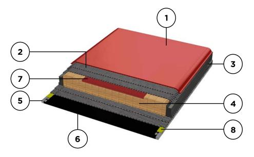
The best compromise between flex and torsion. Composed of double layer multiaxial fiberglass, the objective is to make this ski effective in all types of snow. Based on the legendary H-112, having proven themselves on the feet of our best riders, the heavy duty construction gives skiers maximum safety and reliability. Lightweight for more float but rigid to enjoy the most out of tracked out snow, this construction gives you grip in the toughest of conditions!
